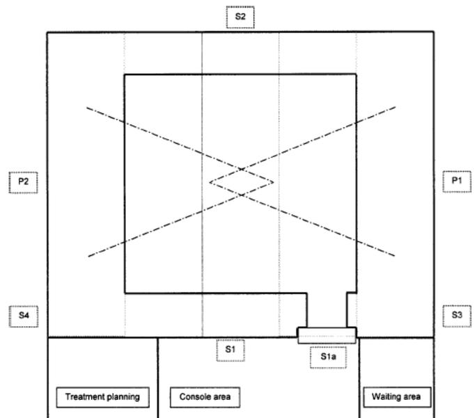
FIG. 2. Plan view of structure. Solid lines are finished walls; light gray dashed lines represent boundaries of modular sections; dash-dot lines represent beam limits. The area designations correspond to Table 1.
